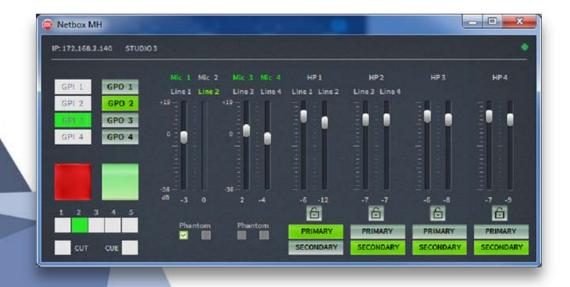
IP audio interface with microphone / line inputs and headphone + line outputs Features general-purpose and radio booth signaling GPIOs
