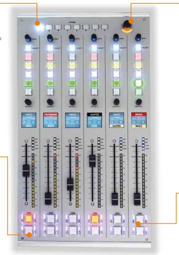
Next to the page swap keys, there is a touch & turn rotary encoder to perform precise adjustments on the touch screen.
